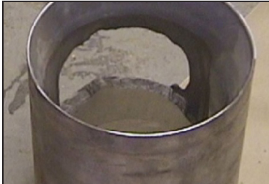
Chrome liner after only 3 months operation
